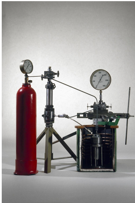
Fig 1 : Apparatus used to discover polyethylene, 1933
